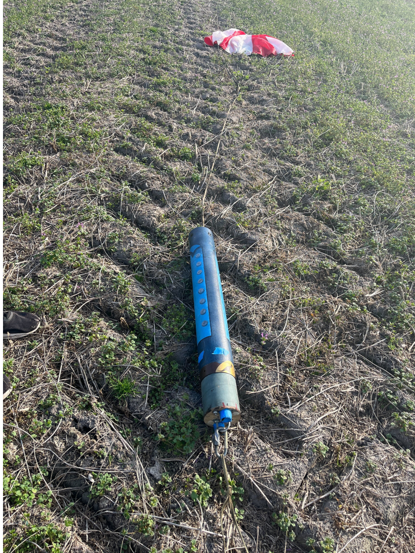
Figure 3.38: Main Parachute/Payload Bay Landing Configuration
