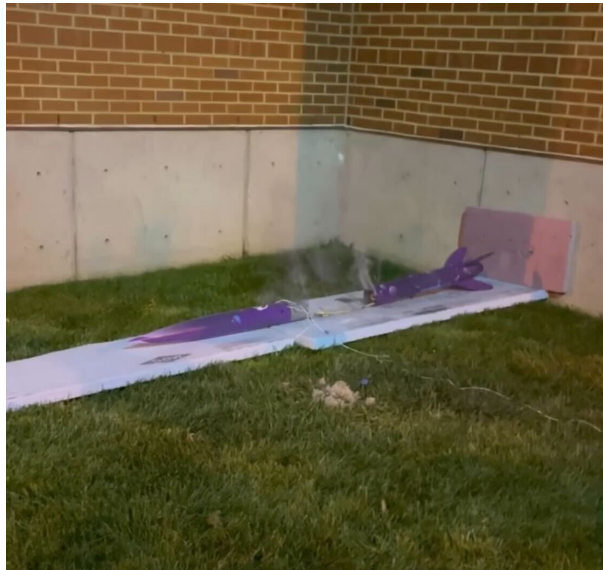
Figure 114: The subscale vehicle just after ejection test of the drogue deployment.
