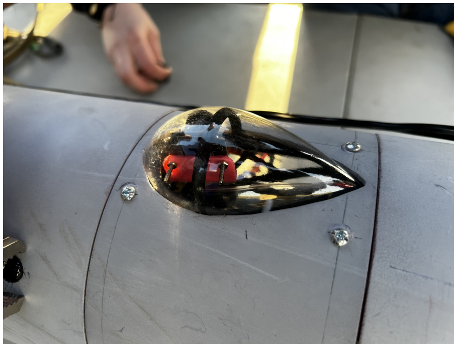
Figure 131: The full camera system assembled to receive APRS commands.
