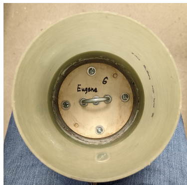
Figure 6: Nose cone bulkhead while installed in the nose cone.
