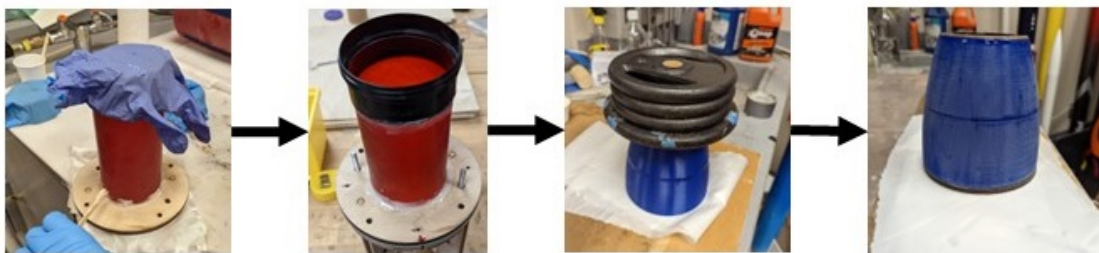
Figure 33: Diagram of the thrust plate and tail cone manufacturing process.
