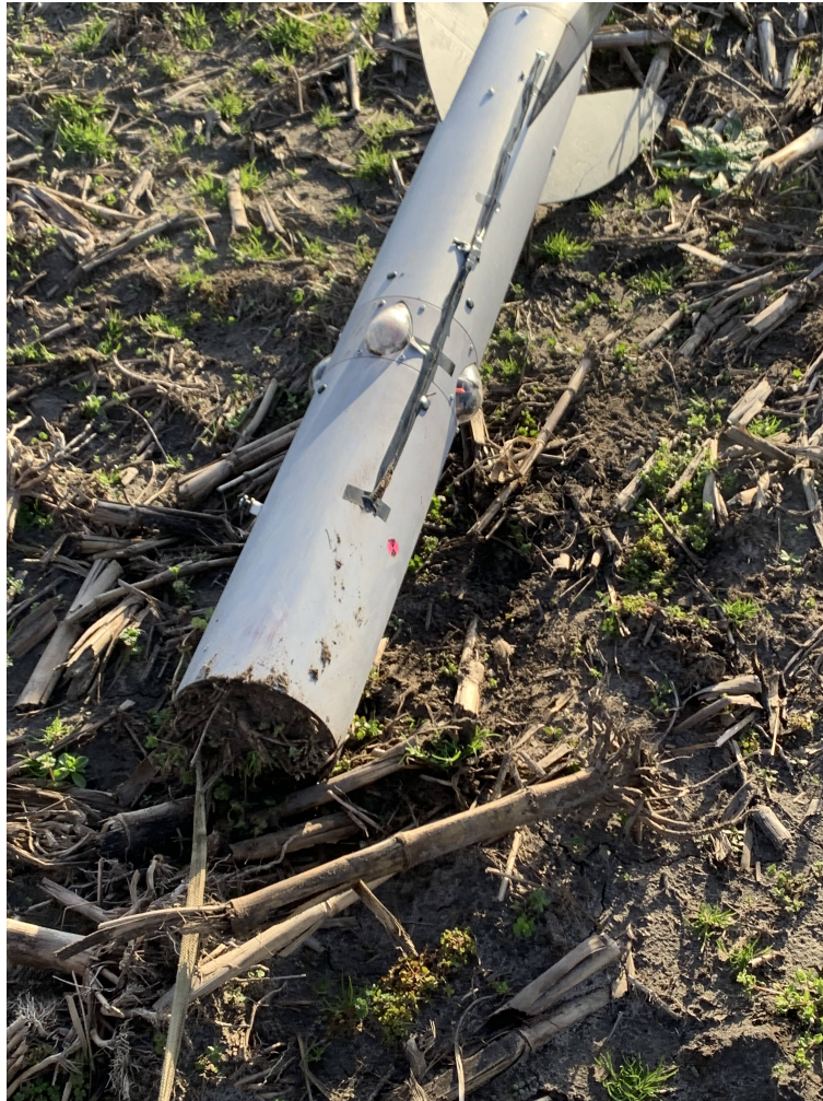
Figure 113: The fin can and payload bay immediately after landing.
