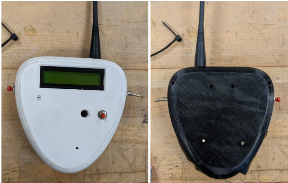
Figure 43: Eggfinder LCD Receiver in its 3D printed case
