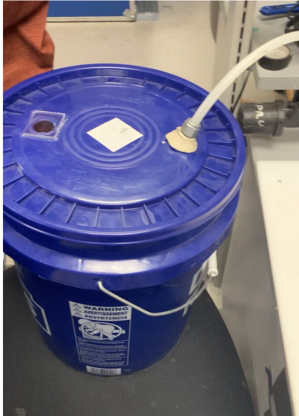
Figure 117: The vacuum chamber for altimeter testing
