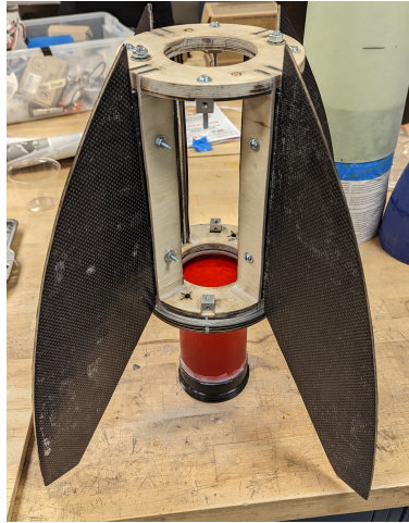
Figure 18: Removable fin assembly.
