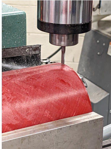
Figure 32: Fin slots being cut on the milling machine.
