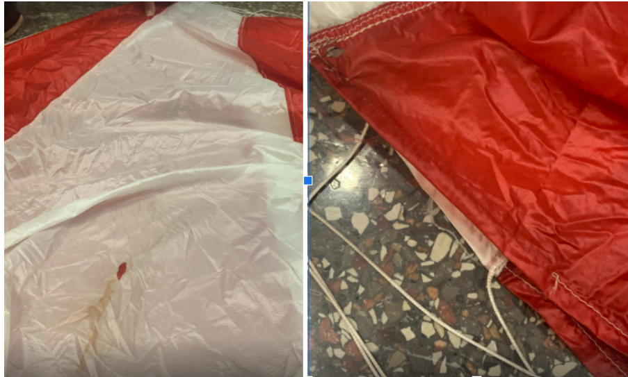
Figure 111: Parachute damage during demonstration flight
