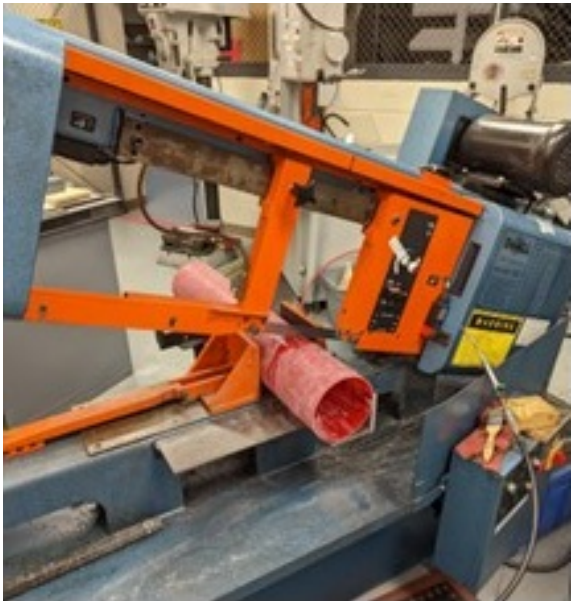
Figure 27: Drop band saw used to cut airframe.
