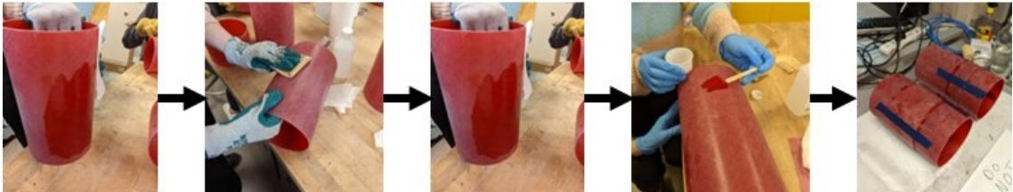
Figure 28: Diagram of the process of cutting and bonding of airframe sections.
