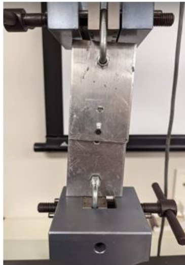
Figure 122: Shear pin testing setup.
