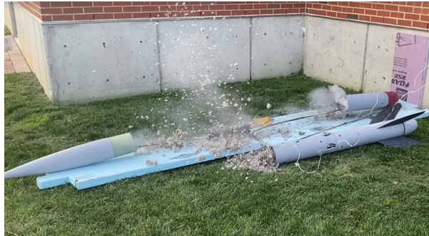
Figure 127: Full scale ejection of the main parachute ejection charge.
