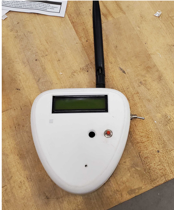
Figure 116: The handmade GPS receiver used for testing.
