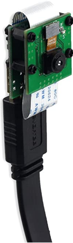
Figure 99: A CSI to HDMI adapter is affixed to the rear of each camera, allowing HDMI output.
