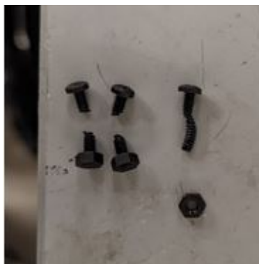
Figure 123: Results of shear pin testing.
